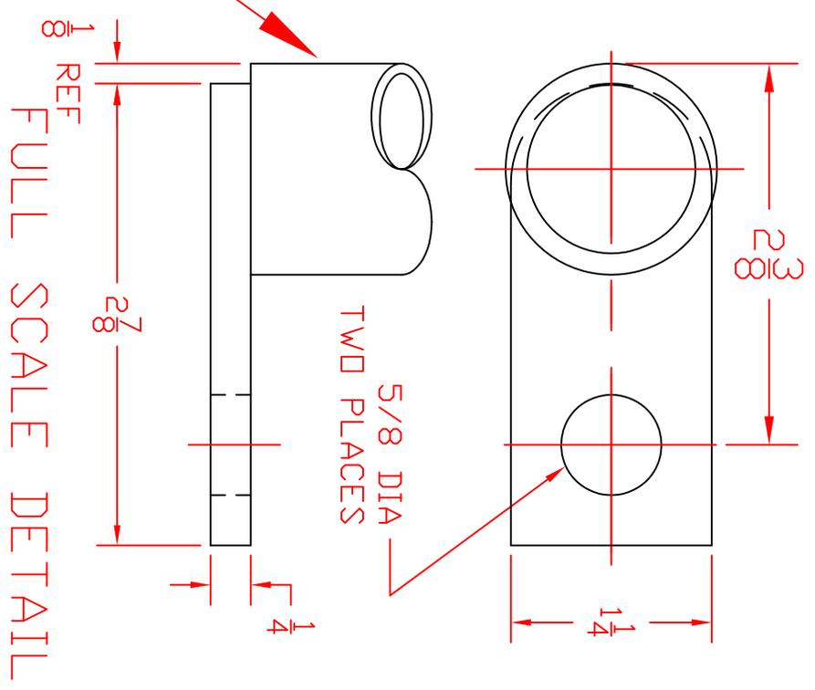
NOTE: WELD WITH LOW HYDROGEN ROD
